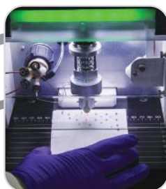
Plate Express ™ : TLC/CMS Mass Analysis of TLC spots
